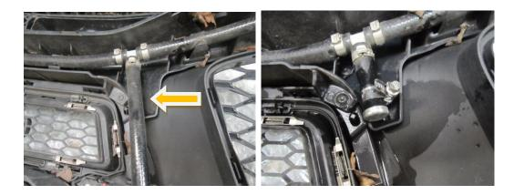
28. You must now tighten up the M8 allen cap bolts that hold the new charge cooler radiator in place, slide the radiator down towards the lower cowling leaving approx 1-3mm gap then fully tighten the radiator in place.
