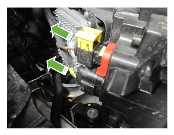
14. Remove the Air temp sensor from the crash bar and disconnect from the wiring loom .
