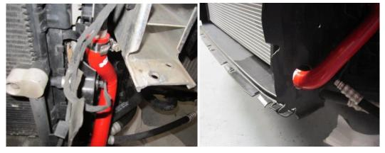
23. You must now remove the upper chargecooler hose fully ,this is arrowed and pictured below.
