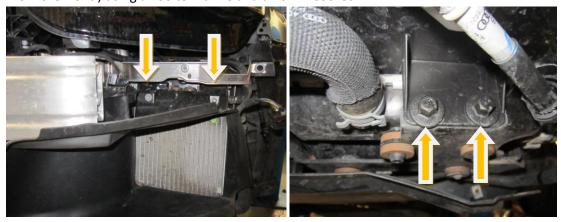
12. Using a T30 torx drive loosen the fasteners that hold the head light in place. The fasteners that are arrowed red must be removed fully .
