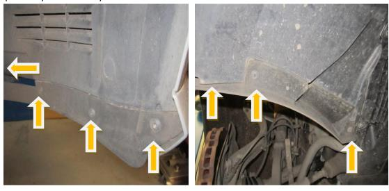
6. Using a T25 Torx drive, remove the two fasteners that join the front corner of the bumper to the arch.
