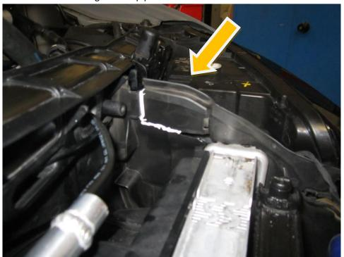
21. Where the lower Forge Motorsport charge cooler radiator pipe sits, a 40 mm hole must be drilled in the cowling as per the picture below .
