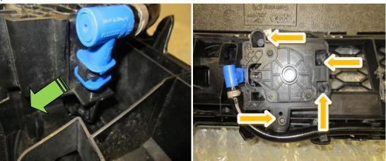
27. Taking care with a sharp knife cut the washer jet pipe as pictured below then insert the 10mm blanking plug and secure it in place with the hose clamp provided.
