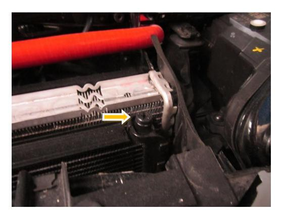
31. Keep checking the coolant level until fully bled .
