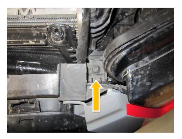
9. For the removal of the front bumper, it is advised you have help so that while one person pulls the bumper towards them they can then hold the bumper still whilst the other can disconnect various plugs on the wiring loom including the washer jets.
