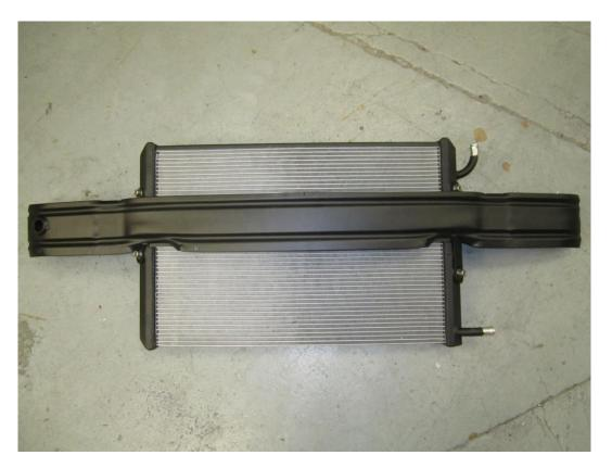
18. We found it helped to pry the crash bar mounts open slightly before loosely mounting the new Forge Motorsport chargecooler radiator in place.
