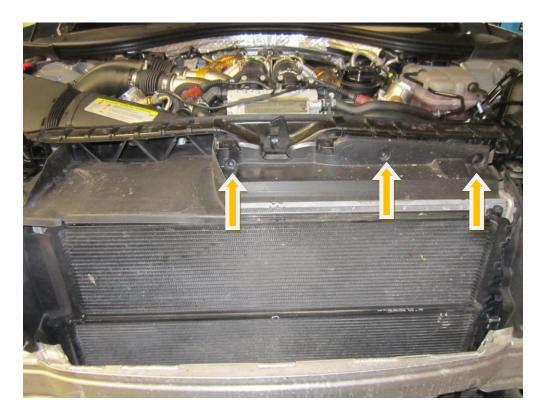
11. Remove the auxiliary radiator ducting on the right hand side of the vehicle (when viewed from the front ) using a T30 torx drive and a 10mm socket.
