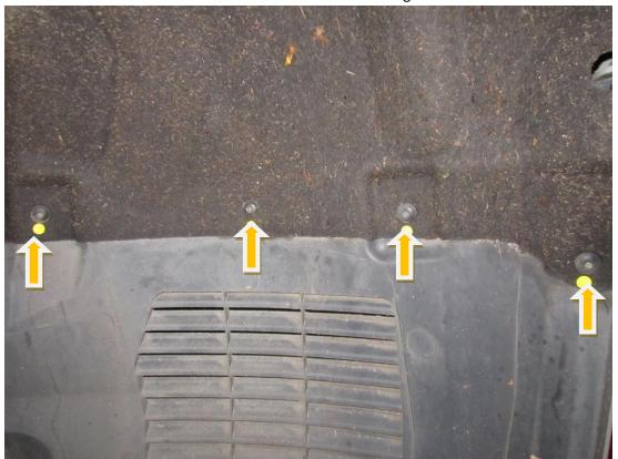
5. Again with your T25 torx drive remove the 7 fasteners that hold the lower arch spoiler in place to your undertray and arch liner.
