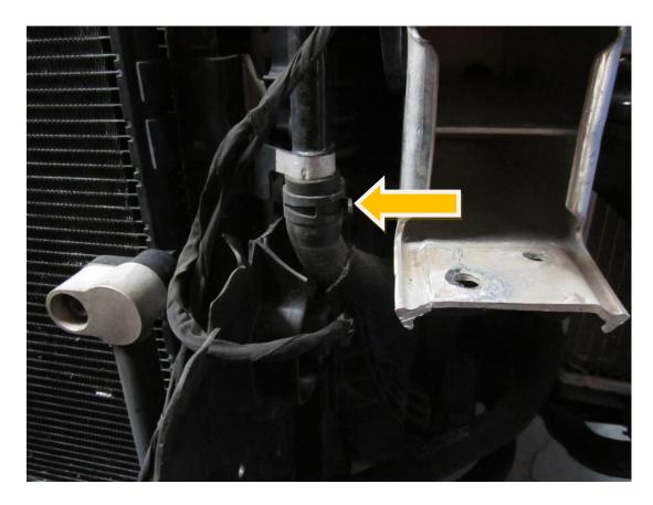
20. Trim part of the cowling with a sharp knife as shown in the picture below. This is to enable space for a new silicon charge cooler pipe .
