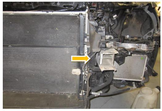
17.Fit the new forge motorsport radiator to the modified crash bar provided. Do not tighten the M8 allen caps fully as there is adjustment that is needed in a few further steps.
