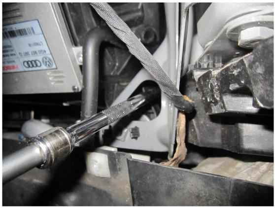
8. Using a T30 Torx drive remove the fastener that holds the bumper in place next to each front headlight .
