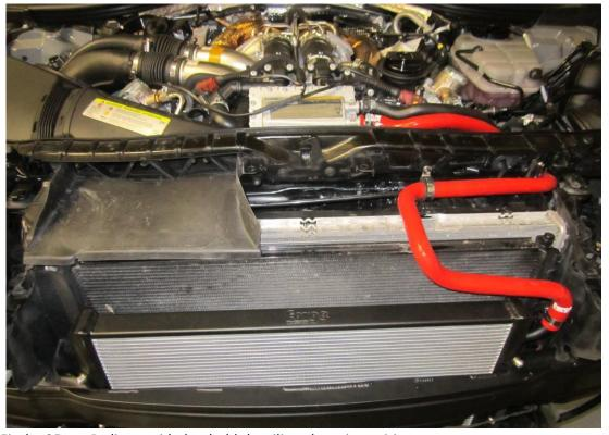
25.Fit the 25mm P-clip provided to hold the silicon hose in position.
