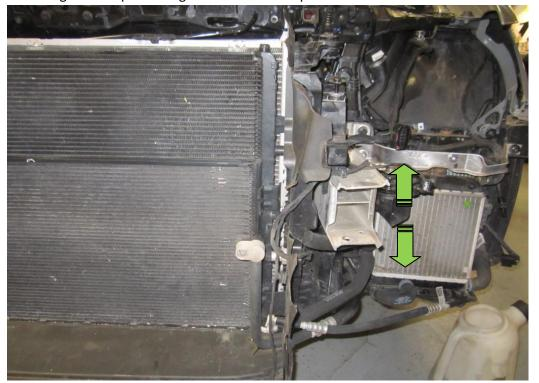
19.Remove the lower charge cooler hose arrowed in the picture below. You will lose the coolant within your OEM charge cooler radiator, so a clean container is advisable to catch this in to either re-use or dispose of correctly.
