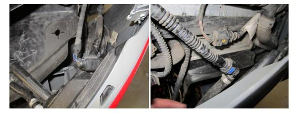
10. Remove the right hand part of the ducting (when viewed from the front of the vehicle) pictured below using a T30 torx Drive. This part can be discarded as it is not needed any more.
