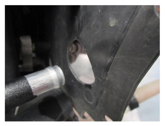
22. Fit the new Forge Motorsport silicon lower charge cooler hose into position and tighten the hose clamps at both end .
