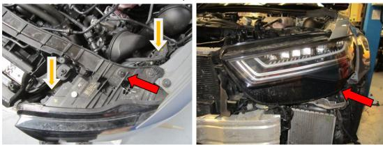
$13. \mbox{Disconnect}$  the wiring loom from the back of the headlights then fully remove .
