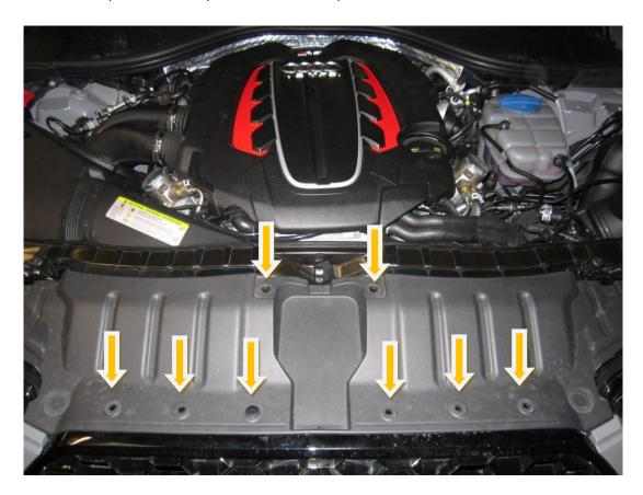
3. Using a T30 Torx drive remove the 4 Torx fasteners that hold the undertray in place .
