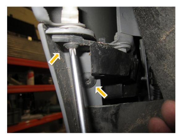
7. Using a 10mm socket and long extension, undo the 10mm hex head that holds the bumper to the front slam panel under the headlight .
