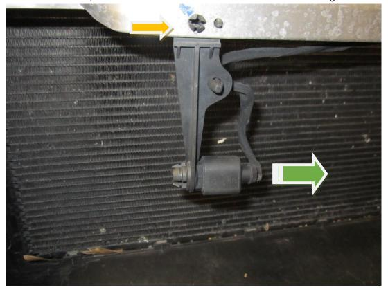
15.Using a 13mm spanner and socket, remove the 13mm bolts either side of the crash bar that hold it in place, then fully remove.
